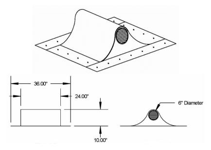
DCSM Off-Ridge Roof Vent - T Minimum 26 ga. ASTM A792 AZ50 or ASTM A653 G90 steel; Maximum dimensions of the vent are 36-inch wide x 42-inch long x 10-inch high. Material shall conform with FBC Section 1507.4.3
